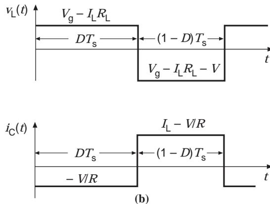
**Figure 5.** A nonideal boost converter: (a) schematic, (b) inductor voltage and capacitor current waveforms.
