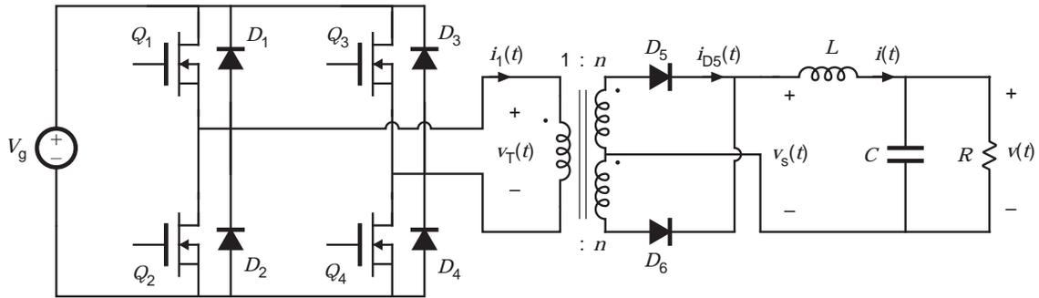
Figure 9. The full bridge transformer-isolated buck converter.
