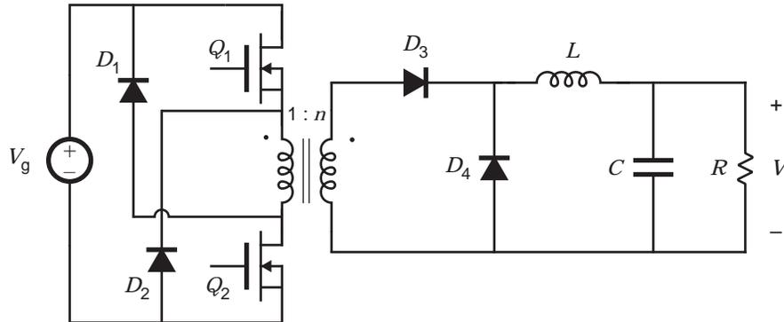
**Figure 12.** A two-transistor version of the forward converter.
