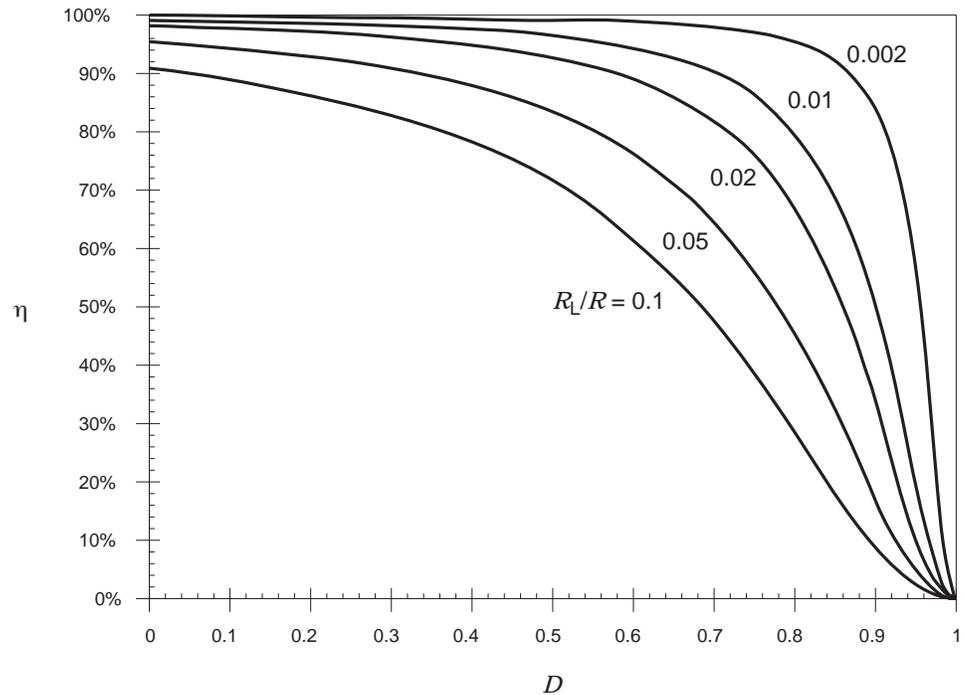
Figure 7. Efficiency vs. duty cycle, for the nonideal boost converter of Fig. 5.
