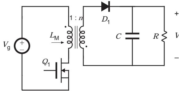
**Figure 13.** The flyback converter, a single-transistor isolated buck-boost converter.
