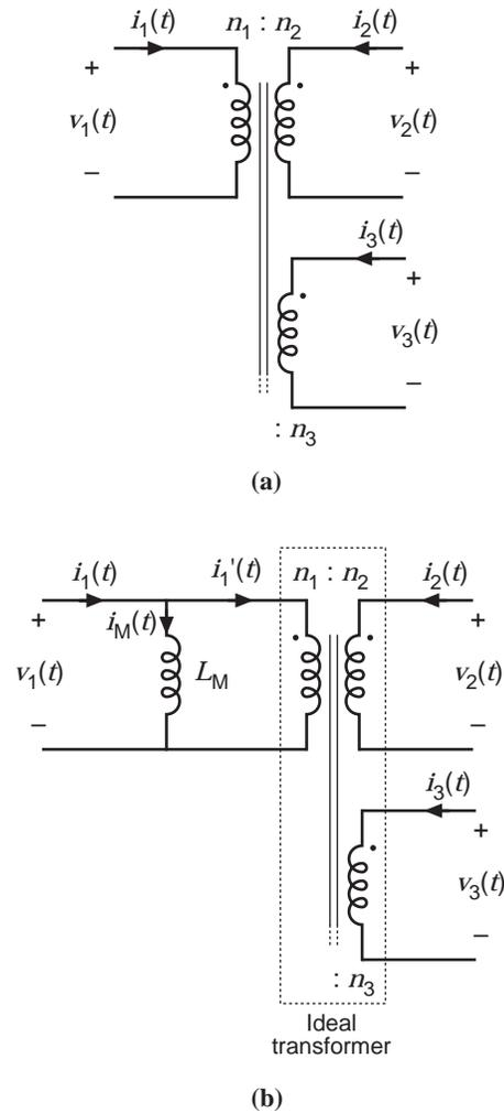
**Figure 8.** Modeling a physical transformer such that its basic operation within an isolated dc-dc converter can be understood: (a) transformer schematic symbol, (b) equivalent circuit model that includes magnetizing inductance  $L_M$  and an ideal transformer.
