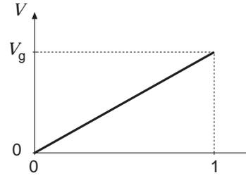
**Figure 2.** Buck converter dc output voltage  $V$  vs. duty cycle  $D$ .
