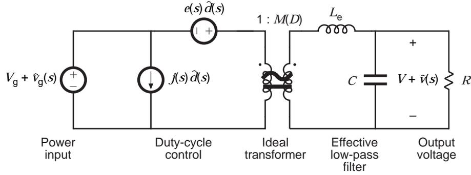
**Figure 15.** The canonical model: a small-signal equivalent circuit that models dc-dc converter dynamics and transfer functions.
