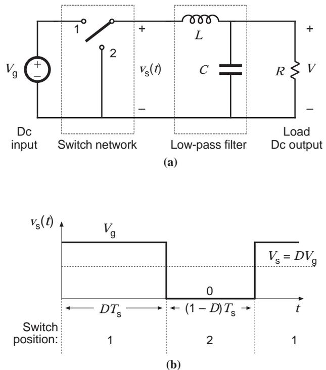
**Figure 1.** The buck converter consists of a switch network that reduces the dc component of voltage, and a low-pass filter that removes the high-frequency switching harmonics: (a) schematic, (b) switch voltage waveform.
