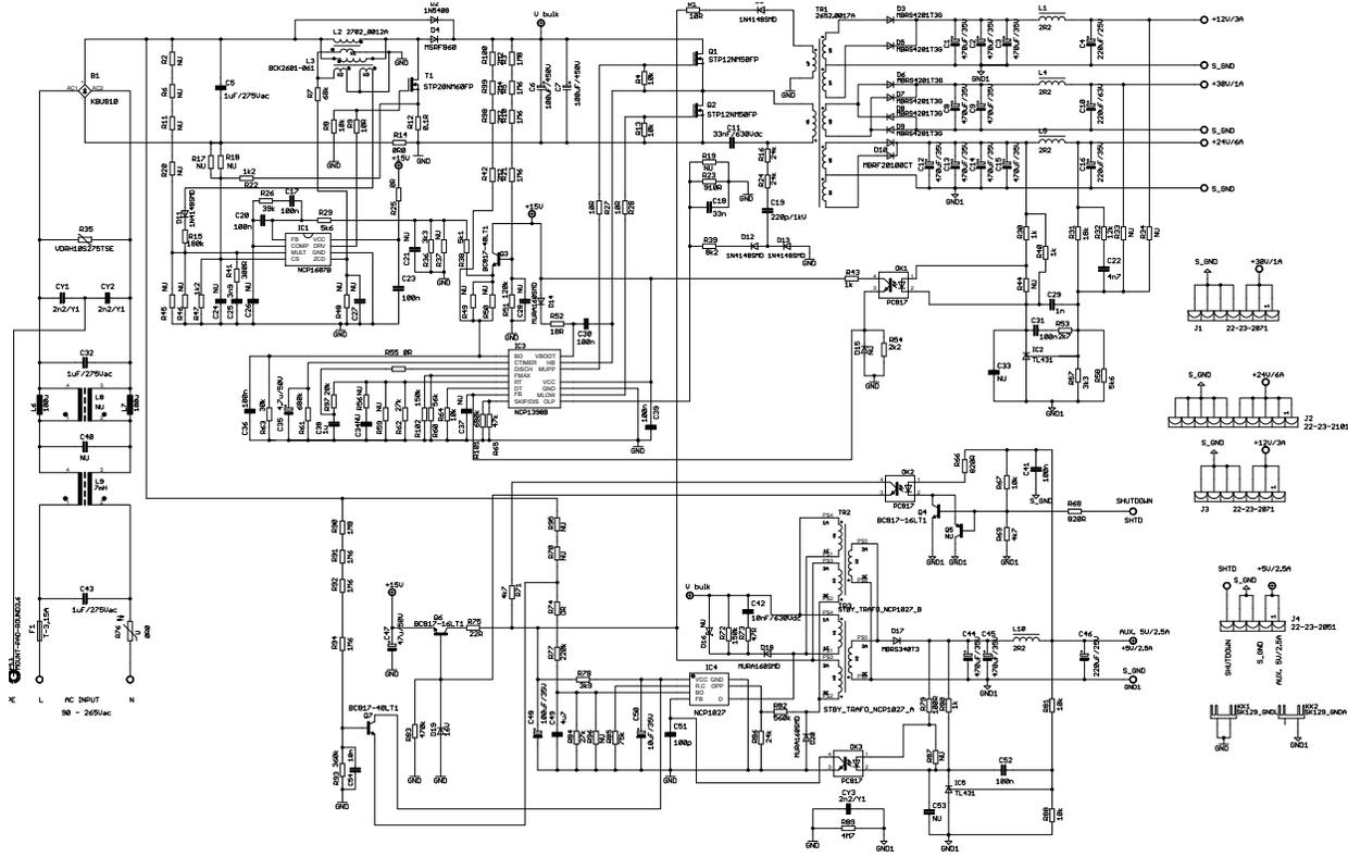
**Figure 47. 220 W LED-TV Design Power Supply**
