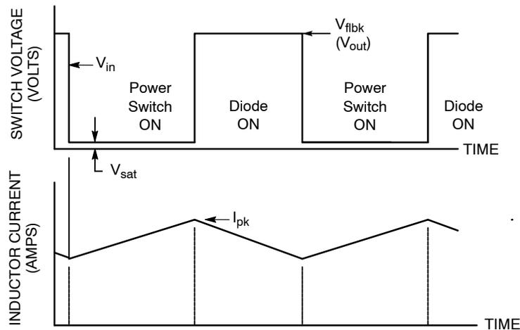
Figure 3. Waveforms for a Continuous-Mode Boost Converter
