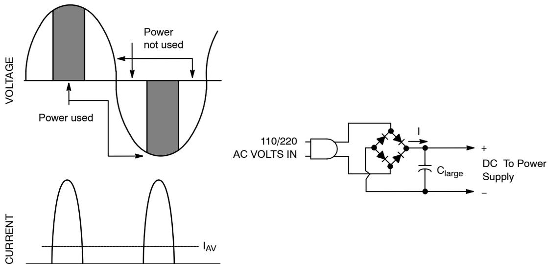
Figure 33. The Waveforms of a Capacitive Input Filter
