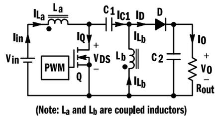
The SEPIC circuit is used when the input voltage must cover a range that is both greater than and less than the output voltage and of the same polarity. As in a boost circuit, the input current is smooth, and the output current (into the output capacitor) is discontinuous. Capacitor ripple current is large.
