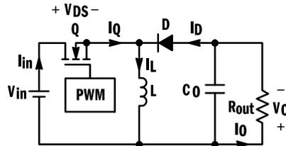
The inverting buck-boost converter is used when the absolute value of the output voltage is greater or lesser than the applied input voltage and the user wants a negative output voltage.
