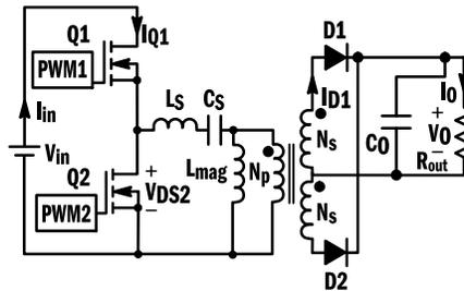
It offers high efficiency and requires no inductor at the output. However, it has high ripple current in the output and is difficult to be operated at light loads.
