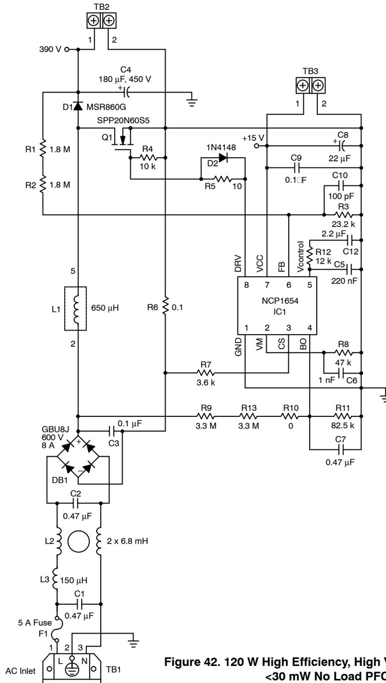
Figure 42. 120 W High Efficiency, High Voltage, Active X2, <30 mW No Load PFC
