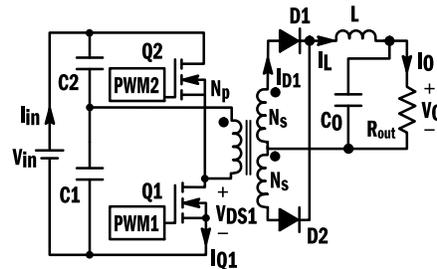
Half-bridge converter is used at medium power levels in the range of 200-700 W for step down applications. It has lower part count when compared to the full-bridge converter but the transistor switches have to handle twice the current compared to a full-bridge converter.
