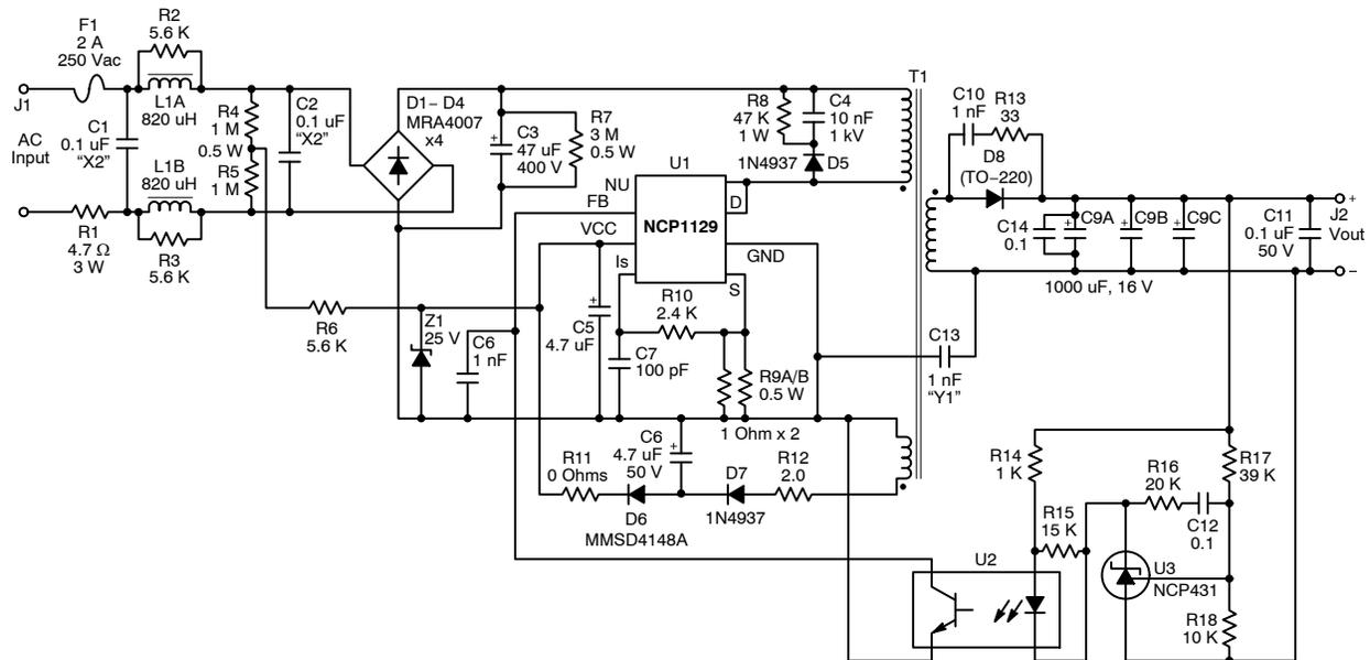
Figure 44. 25 W Offline Power Supply High Voltage Switcher
