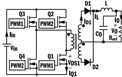
A full-bridge converter is used at high power levels in the range of a kW and is normally not used at lower power levels due to its higher part count. It is normally used in step-down applications.
