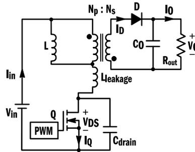
This topology is used at power levels which are lesser than 150 W. It allows operation at variable frequencies.
