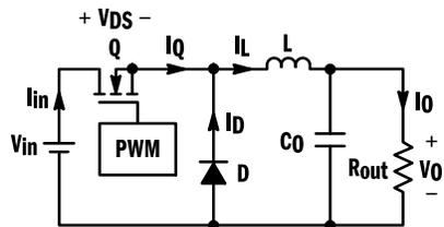
The buck converter is used when the required output voltage is less than the input voltage. When the output voltage requirement is low, the diode D is replaced by a switch which is called a synchronous rectifier.
