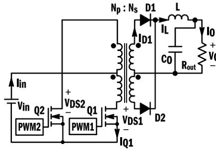
Push-pull converter is used when there is a wide variation in the input and when the output voltage is lesser than the input voltage. It can be used at power levels in the range of few hundred watts to 1 kW.
