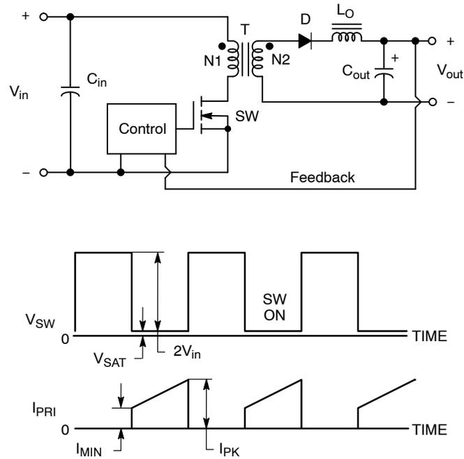
Figure 9. The One-Transistor Forward Converter (Half Forward Converter)
