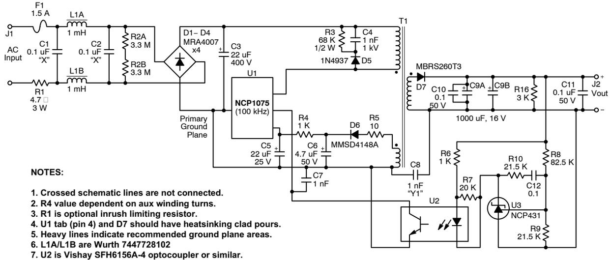
Figure 43. Up to 15 W AC–DC Compact Power Supply
