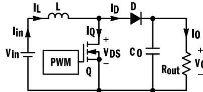
The boost converter is used when the required minimum output voltage is greater than the maximum input voltage. It can be used in Continuous Conduction Mode (CCM) to minimize the peak current or in Discontinuous Conduction Mode (DCM) to minimize the inductor value. It is also employed as a pre-converter for Power Factor Correction applications.
