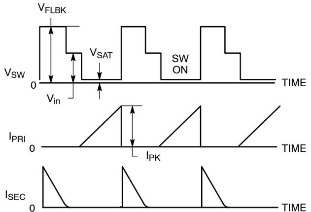
**Figure 8. The Flyback Converter**
