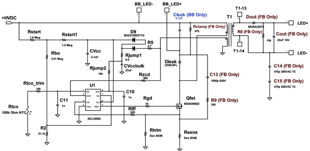
NOTE: Components labeled **FB** are only populated for the flyback version and components labeled **BB** are only required for the Buck-boost configuration
