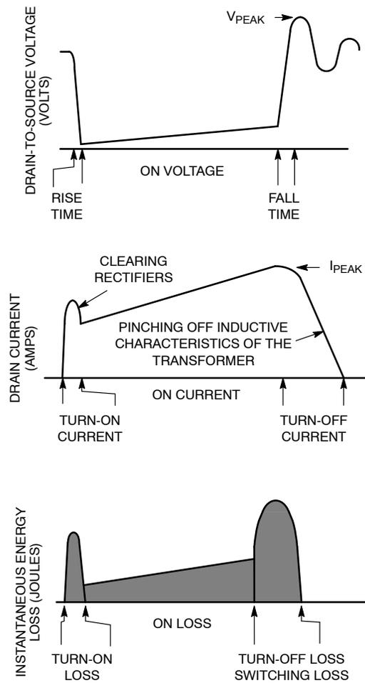
**Figure 24. Stresses and Losses within a Power MOSFET**
