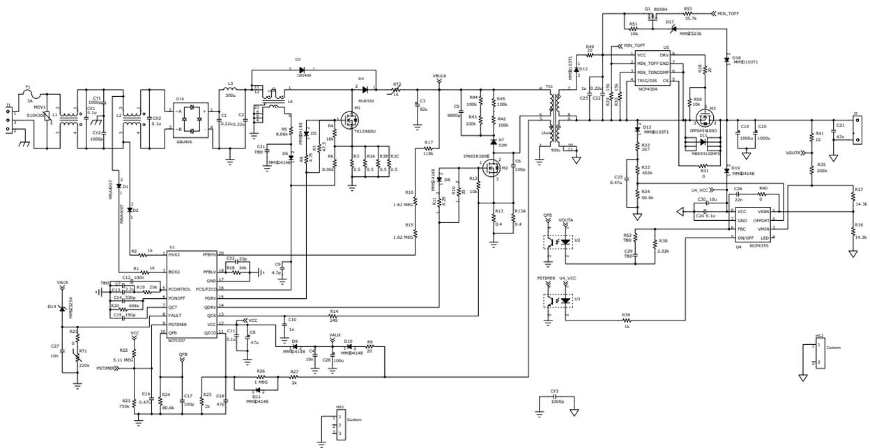
Figure 48. High Efficiency 90 W SMPS Based on NCP1937
