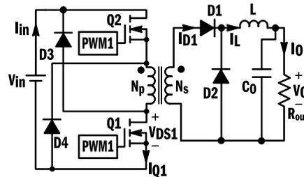
Two-switch forward converter, a variation of the forward converter can be used at higher power levels and does not have an additional reset winding. The voltage stress on the switches is less in this case when compared to a single switch forward converter.
