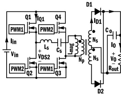
It offers high efficiency and requires no inductor at the output. However, it has high ripple current in the output and is difficult to be operated at light loads. Full-bridge version provides two times higher gain compare to half-bridge resonant topology and is usually used for high output power.
