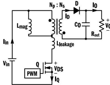
The flyback converter, derived from the buck-boost converter is normally used at power levels below 150 W. It has a higher switch rating due to the reflected output voltage appearing across the switch in addition to the applied input voltage. It is also used for Single Stage Power Factor Correction applications.
