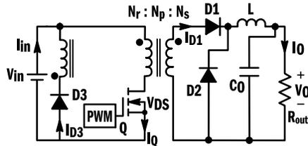
The forward converter, derived from the buck converter is used at power levels typically in the range of 150 - 400 W. It is widely used for step down applications.
