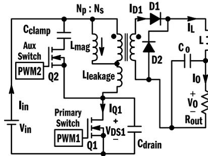
It is normally used at high power levels in the range of few hundred watts. It has a higher parts count and requires a dedicated controller, but offers a higher efficiency due to soft switching. It can tolerate wide input voltage variations.
