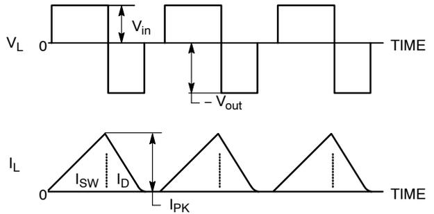
**Figure 7. The Buck-Boost (Inverting) Converter**
