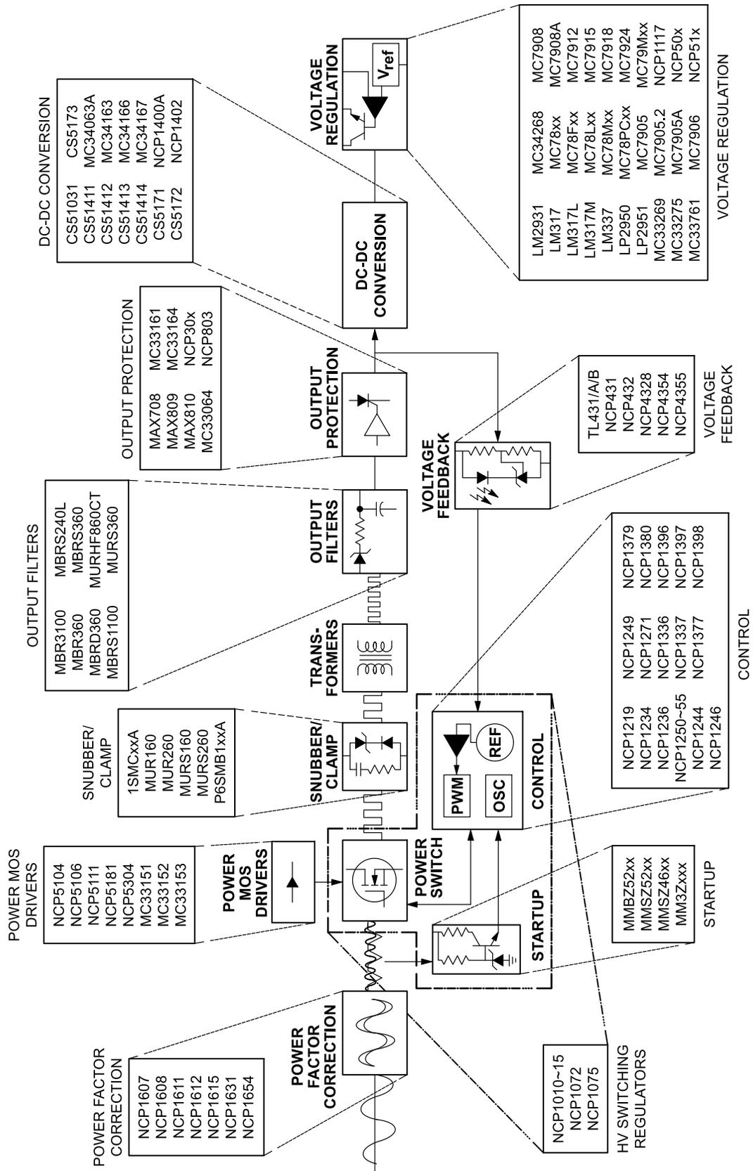
Figure 36. Integrated Circuits for Switching Power Supplies
